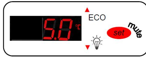
Face of alarm/thermostat
