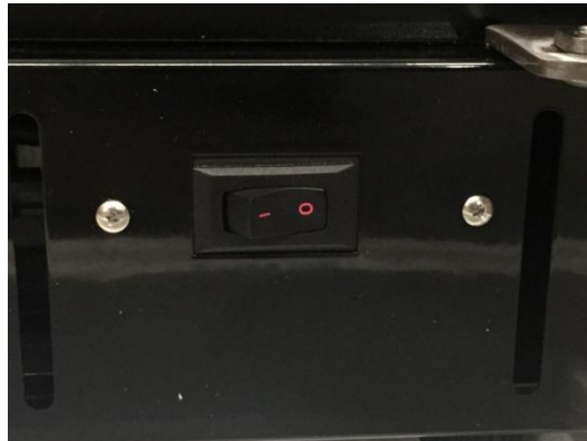
Power switch located in kickplate on the right side
