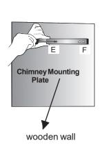
Screw the chimney mounting parts into Ø 8mm sized wall plugs on E,F points which are provided with your product.
